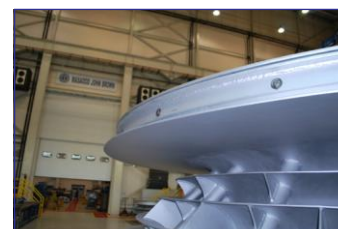
Adjustable aft sealing ring
